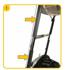
Install provided plastic extrusions onto the front roof struts from the inside of the cart. The protruding ribbed flange is positioned on the outside of the strut facing the rear of the cart. Two pieces of the 11 inch long extrusions get installed on each side of the cart above and below the windshield hinge. Align the holes in the plastics with the windshield bolts and press onto the struts.
