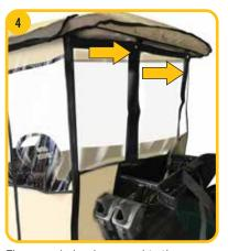
The rear window is secured to the cover with two snaps along the upper edge of the window. The sides of the window are zippered onto the cover. If the rear window is installed with the Cabana Bag Cover, it is placed inside of the roof struts and then secured to the top with the snaps and zippers as stated previously. The 3-Sided installation is complete.
