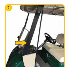
Install the front fabric panel onto the previously installed plastic extrusion by pressing the rubber extrusion onto the ribbed flange. Wrap the fabric straps around the windshield struts and secure with Velcro. Press rubber extrusion onto the front wheel lip of carts body.
