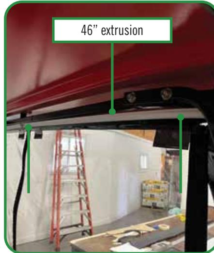
Using the 46" rail, align the rail along the canopy support rail. Drill the first hole to utilize the factory canopy bolt 1 3/4 back from the forward edge of the rail. This rail will also utilize the center factory canopy bolt. Repeat on opposite side of the cart.
