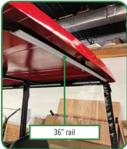
Using the 36" rail, center rail on the rear canopy support bar. Mark the rail to drill a hole to utilize the center factory canopy bolt. Mark and drill each end of the 36" rail to drill and transfer drill holes into the factory canopy support using a 3/16 drill bit. Secure rail the cart using the center factory bolt and thread forming screws.
