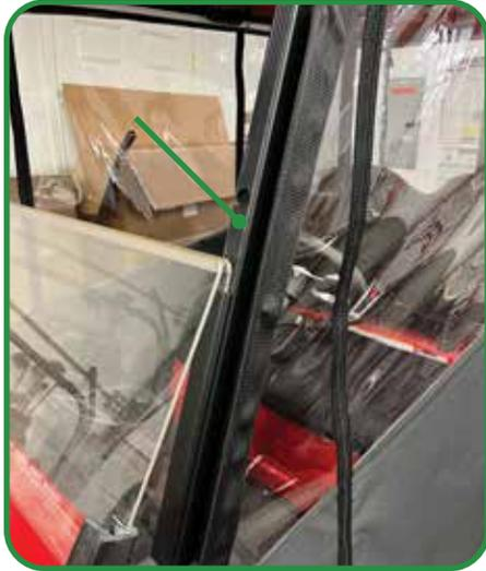
Remove factory windshield extrusions and replace with the provided extrusions. Re-install windshield.
