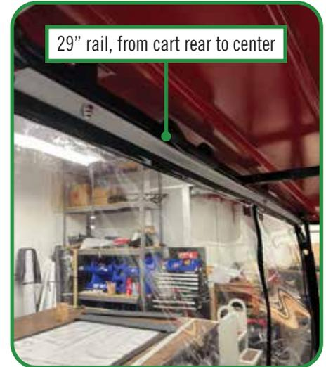
Using the 29" rail, align the rail with the previously installed forward rail along the canopy support. Mark and drill a hole to utilize the rear factory canopy bolt. Mark and drill the forward edge of the rail and transfer drill a hole into the factory canopy support with a 3/16 drill bit. Secure using a thread forming screw. Repeat on the opposite side of the cart.
