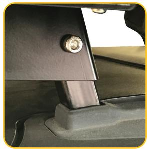
Secure the bracket to the sweater basket support strut. Insert the supplied M8x40 bolt into the bracket and through the lower factory hole on the sweater basket support strut. Secure on the back side of the strut with the M8 washer and M8 lock nut.
