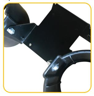
Attach sand bottle holders to the right and left side of the Iron Maid bracket using the supplied M6x15 bolts with a washer under the head and nylock nuts.
