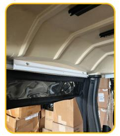
Center the 18-inch rail on the inside of the "tab" on the inside of the canopy and mark holes for drilling approximately 2 inches from each end. Drill ¼ holes at each marked location. Transfer drill holes from the rail into the tab. Secure the rail with the bead facing inside the cart with the supplied M6x20 bolts with flat washers under the head and the M6 nylock nuts.
