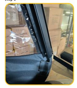
Secure the front panels to the new windshield extrusions by pressing the rubber channel onto the tab on the backside of the extrusion.
