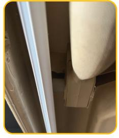
Rear grab handle bolt with ½ spacer between rail and handle.
