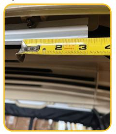
Front canopy bolt with 3 inches of rail forward of the bolt.
