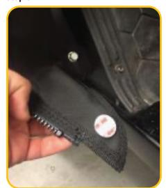
Attach the adhesive snap onto the snap on the front panel. Use the panel to approximate the location the snap will attach to the rocker panel. Clean the rocker panel and allow to dry. Apply the 3M adhesive primer to this area and allow to dry. With the snap still attached to panel expose the adhesive backing and set in place using the panel as a locating guide. Keep pressure on the snap for 60 seconds. Allow the snap adhesive to set for 24 hrs. without disturbing.
