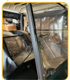
Replace the factory windshield extrusions with the new supplied parts, secure with factory hardware.
