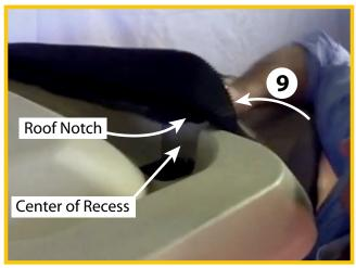
**9.** Align bracket with roof notch at center of recess and press firmly to snap in place (2 places).
