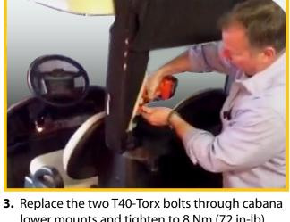
lower mounts and tighten to 8 Nm (72 in-lb).
